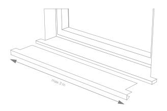
3 Clean the substrate to remove dust and apply the installation glue. Slide the overlay onto the old windowsill.
