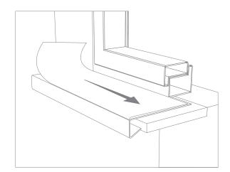
6 Fill the gap between the sill and the wall using silicone.
