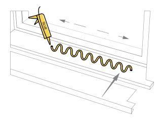
Fix the end caps of the overlay using an instant glue (e.g. "Super Glue").
