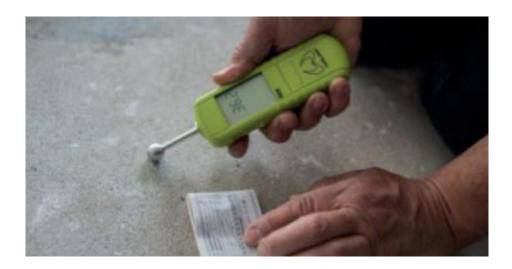
The moisture content of the underlying surface should be in accordance with local or national standards for the installation of resilient floor coverings. If in doubt, seek further professional advice.
